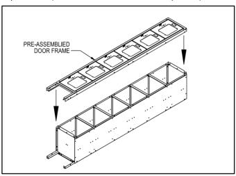
**Step 5:** Tighten all fasteners, ensuring the locker remains square during the process. If desired, attach optional sloping hood, end bases, or front base (see pages 4 and 5).
