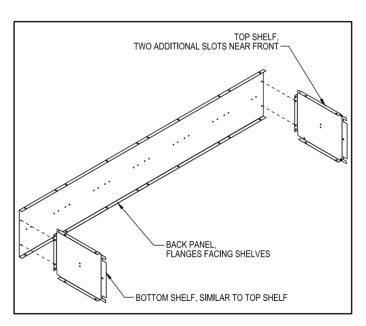
**Step 2:** Turn the back panel onto its back with the shelves pointing upward. Attach the first side panel, the left rear leg, and five compartment dividers to the assembly from Step 1.
