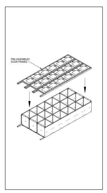
**Step 9:** Tighten all fasteners, ensuring the locker remains square during the process. If desired, attach optional sloping hood, end bases, or front base (see pages 4 and 5).
