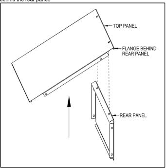
**Step 2:** Attach the side panels to the top panel and rear panel. Sloping hood assembly is now complete.
